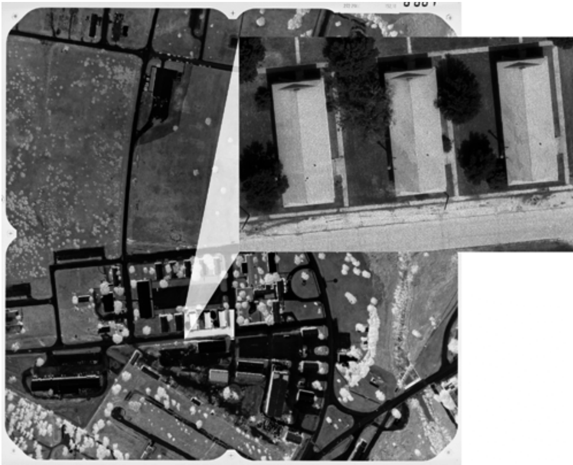
Figure 9 : Scanning of black/white negative film (shown in the background) and an enlarged section of high contrast, scanned at 25 \mu\text{m} pixel size (note the details in the bright area as well as in the shadow).
